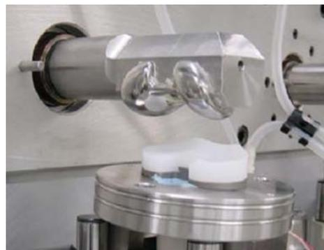
**Fig. 1** Knee simulator test (AMTI-Boston 6 Station Knee Simulator, AMTI, USA). Ti-6Al-4V alloy (NAKASHIMA propeller) was used as femoral component and Hi-tech Knee II (Total Knee System, NAKASHIMA Medical, Japan) which has flat surface geometry, was used as tibial component.
