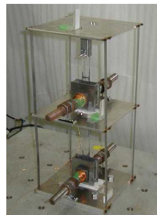
Fig. 9 2DOF model with MR damper
