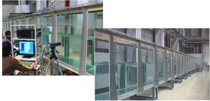
Figure 5: Wind-wave tank (30 m long and 0.6 m wide) installed at the Fluid Dynamics Advanced Research Institute. This tank is used to study turbulent structure and heat and mass transfer at the gas-liquid interface.
