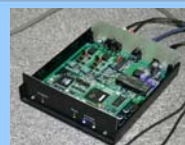
DA converter with YY filter implemented on TI C6713 DSP
